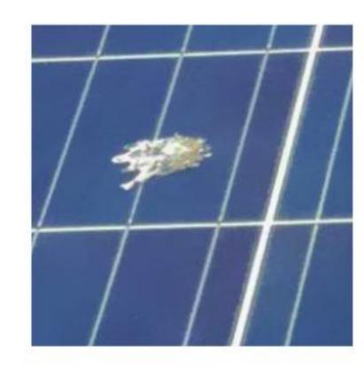
Impact of pollutants, dust, bird droppings, rust, etc. on power generation efficiency.
